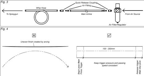
Fill the paint cup with the appropriately thinned paint and screw onto the gun. Connect the air hose switch on compressor. See *Fig. 3* for the recommended air line setup. It is recommended that you use a test card or scrap panel to make sure that the paint is correct. This also aids comparison with existing paint work.
