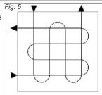
Never start or stop the gun whilst it is aimed at the workpiece. Too fast a pass will give a thin and patchy coat whilst too slow a pass will result in a heavy coat. Apply one coat at a time and observe manufacturers drying times before applying the next coat or finishing/polishing.
