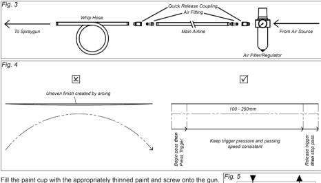
Connect the air hose switch on compressor. See Fig. 3 for the recommended air line setup. It is recommended that you use a test card or scrap panel to make sure that the paint is correct. This also aids comparison with existing paint work.
