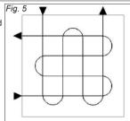
Never start or stop the gun whilst it is aimed at the workpiece. Too fast a pass will give a thin and patchy coat whilst too slow a pass will result in a heavy coat. Apply one coat at a time and observe manufacturers drying times before applying the next coat or finishing/polishing.
