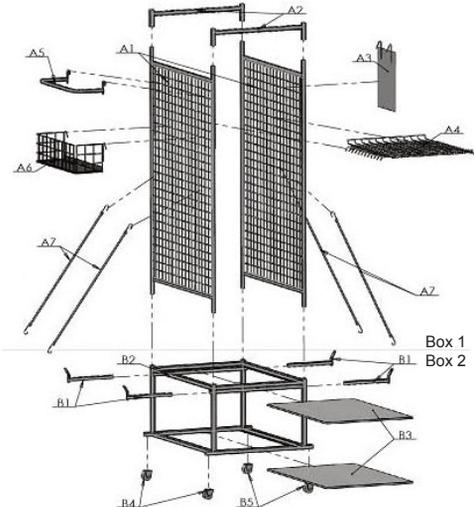
This equipment is designed to be assembled without the aid of extra fixings.
